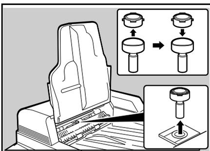
1. Remove by pulling the Stamp Assembly upward.
