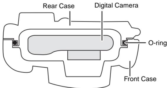
The gum comes into contact with the sides of the Case making the Case waterproof and stopping water from entering from the gap.
