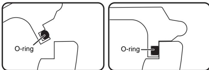
When water pressure acts on the O-ring, the surface of the O-ring expands and the Case is sealed more tightly.
