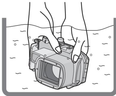
**Carry out the same test after attaching the digital camera to the Case. (P15)**
