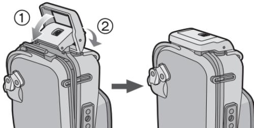
Check that the buckle is closed firmly.
