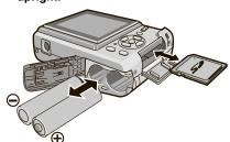
Do not touch the connection terminals on the back side of the card.
