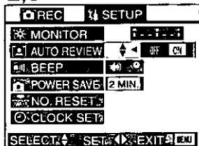
Recording with the auto review set to [ON], the recorded picture is automatically displayed on the LCD monitor for about 2 seconds.
