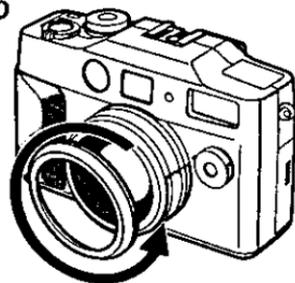
Using the tele conversion lens (DMW-LT52, optional), it is possible to zoom in much more; using the wide conversion lens (DMW-LW52, optional), it is possible to widen much more. (When attaching the conversion lens to the camera, the conversion lens adaptor (DMW-LA1) is necessary)
