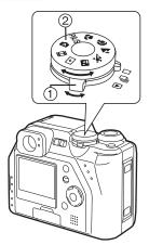
■ Operational mode dial ① With this dial you can set REC (single mode or burst mode) and playback modes.
