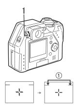
This camera's optical view finder offers a diopter adjustment. It allows the user to make adjustments related to each users individual vision characteristics. Please adjust this feature before using the camera.
