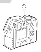
When the card is being accessed, the red flash/access indicator ① lights.
