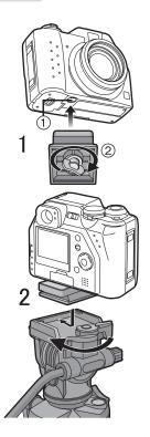
Using a tripod (customer supplied), can minimize or eliminate picture motion jitter associated with physical movement. This is especially true when in the tele position or when using slow shutter speeds.
