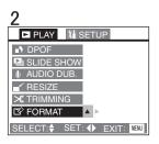
Usually, it is not necessary to format the card (initializing). Format the card when this message is displayed "MEMORY CARD ERROR".
