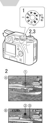
By only pressing the shutter button, the exposure (shutter speed and aperture value) will be automatically adjusted and the picture will be taken.
