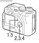
Recording with the auto review set to [ON], the recorded picture is automatically displayed on the LCD monitor for about 2 seconds.
