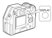
Every time you press the [DISPLAY] button, the display of the LCD monitor changes as shown below.
