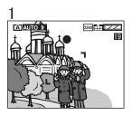
If the subject is out of the AF target or the focus area and you press the shutter button, the subject's focus is not adjusted. After locking focus and exposure (AF/AE lock), you can take a clear picture with adjusted focus. AF: Auto focus
