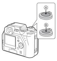
The shutter button is pressed in 2 steps: "pressing halfway" and "pressing fully".
