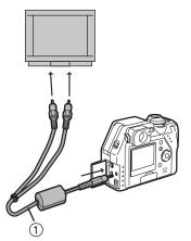
By connecting the camera to a television via the supplied A/V cable ①, it is possible to view and play back the recorded images.
