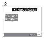
Pressing the shutter button once, the camera will automatically take 3 (or 5) pictures changing exposure according to the set exposure compensation value.
