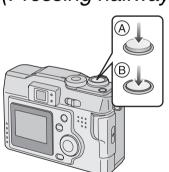
The shutter button is activated in 2 steps: "pressing halfway" and "pressing fully".
