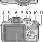
The joystick is operated in two different ways: it can be moved in the up, down, left and right directions to perform an operation, or it can be pressed to select. In these operating instructions, it is pictured as shown in the figure below or described with  $\triangle/\nabla/\blacktriangleleft/\triangleright$ .
