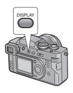
Every time you press the [DISPLAY] button, the display of the LCD monitor/Viewfinder changes as shown below.
