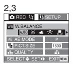
Auto White Balance is designed to automatically adjust the camera to produce natural flesh tones. In most situations it works fine. In some situations where several different types of lighting are present, enhanced performance can be achieved by setting the white balance manually.
