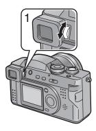
This camera's Viewfinder offers a diopter adjustment. It allows the user to make adjustments related to each user's individual vision characteristics. Please adjust this feature before using the camera. This feature is especially useful for the user who wears corrective eyewear because the lens is not needed.
