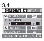
When the shutter speed is set, the aperture value is set automatically according to the subject brightness.
