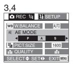
When aperture value is set, the shutter speed is automatically set from 1 second to 1/2000th according to the subject brightness. (However, the speed range is changed from 1/30th to 1/2000th when flash fires.) Altering the aperture value changes the depth of field of the picture.
