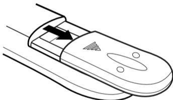
2. Install two "AA" (penlight size) batteries.
