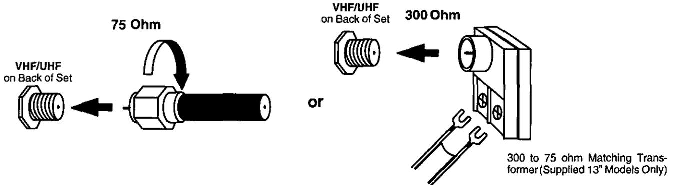
**Cable Connection** – For reception of cable channels, connect the cable supplied by your local cable company. **Antenna Mode must be set to CABLE.** (Refer to Antenna Mode section.)
