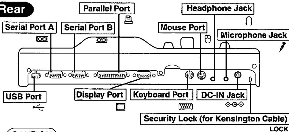
When using the computer with the port replicator, device connectors must be connected to the port replicator, not directly to the computer.
