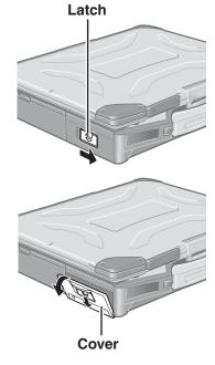
(2) Slide the latch down, and then without releasing it, open the cover as illustrated.
