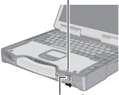
③ Slide the battery pack inward until it is firmly in place.
