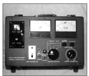
Figure 11 - Toshiba Portable Vacuum Checker
