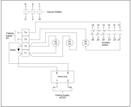
Figure 7 – Internal connection of the latched type
