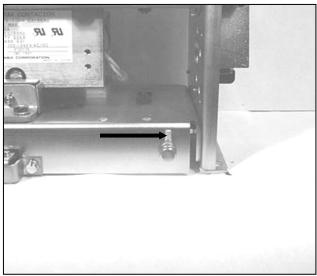
Figure 3 - Ground connection location
