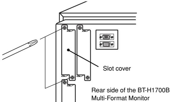
3. Insert the Input Card's board (green-colored) into the slot, fitting the board into the guide rails on the top and bottom of the slot.
