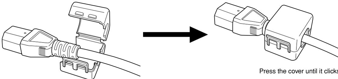
3. Connect the AC power cord to the AC inlet, and join the Power Cord Holder cover with the case.
