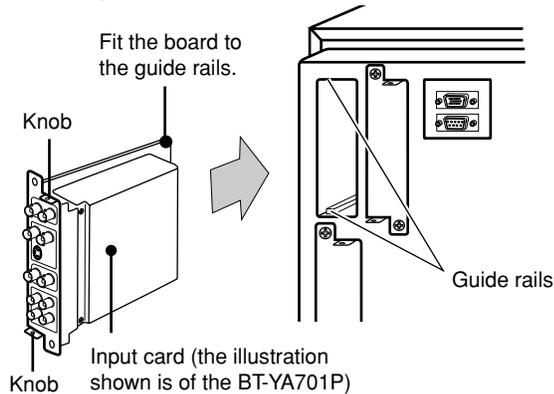
4. Push the Input Card in so that its front panel touches the monitor's rear panel.
