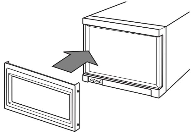
3. Secure the wide mask with the screws (fix 2 screws each to both right and left side).
