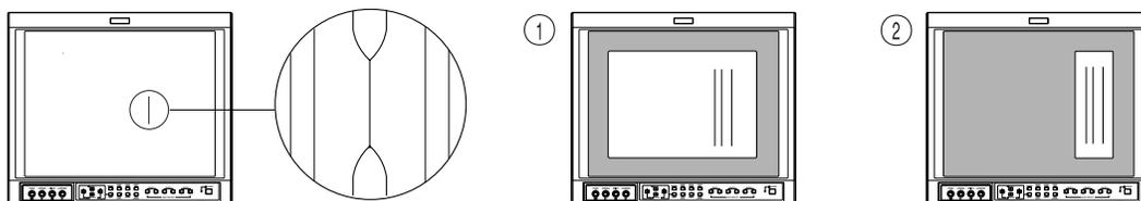
In this case, try tapping the monitor on the side. If this does not get rid of the lines, follow the procedure below.
