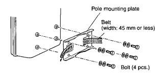
② Fasten the AC adaptor to the pole using the pole mounting plate and the belt.
