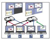
This arrangement can be used when you wish to simultaneously display multiple presentations using multiple projectors.
