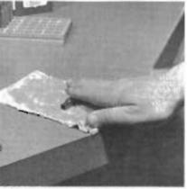
3. Clean, inspect and jubricate cases with pad or rag containing Pacific Case Sizing Lubricant. Do not lubricate excessively or lubricate neck of case as it will tend to wrinkle or buckle case. Under lubrication can cause stuck case in size die.
