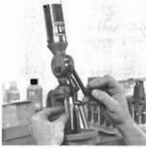
7. Charge case with proper amount of powder using Pacific Deluxe powder Measure or Pacific Powder Scale. Refer to Hornady Reloading Manual or other reliable source to determine proper components and charge for your particular cartridge.
