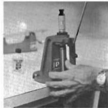
5. With ram in full up position, push primer arm into slot of ram and lower ram so that primer seats in the cartridge case. Care should be taken so that primer is seated fully without applying excessive pressure to the primer. After cartridge is primed, raise ram slightly and return primer arm to original ousition. Exercise care when raising ram so that the deprime punch does not contact new primer and partially deprime case.
