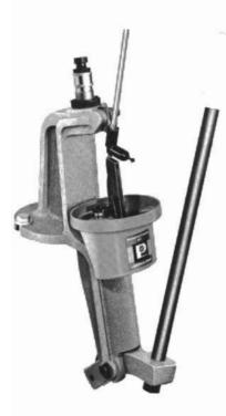
Your Pacific POWER "C"(TM) reloading tool is an improved and strengthened design of Pacific's original patented basic "C" type tool. The heavy duty "C" type frame is of high density cast iron to assure perfect die/shell alignment and take the pressure needed for case forming and bullet swaging.
