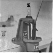
4. Place lubricated case into shell holder and move operating lever down, forcing the ram upwards and the case into the die. This removes the old primer and resizes the case (2-die sets.) With 3-die sets, the resizing and depriming are done in separate operations.
