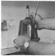
8. Replace size die with bullet seating die and adjust according to die instruction sheet, insert charged case into shell holder and place bullet over mouth of case. Move operating lever down, raising ram upwards and forcing case into die. If die is properly adjusted, the bullet will be seated and case will be crimped. (Pacific bullet seating dies can be adjusted to crimp case or seat bullets without crimping during the seating operation.)
