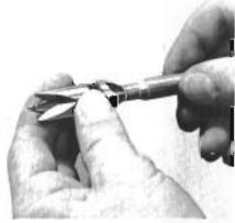
6. Check case length (for cases to be crimped) and trim with Pacific Case Trimmer or File Type Trimmer Die. Chamfer inside and debut outside of case mouth with Pacific Chamfering and Deburring tool, and wipe case free of all lubrication with a clean dry cloth.
