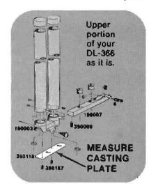
REPLACES MEASURE CASTING PLATE on DL-366 Reloaders mld. 1/68-12/73
