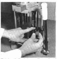
4. Rotate shell plate so that primed and charged case is moved to station #3. With left index finger press down on wad guide bracket (350-51). With right hand place proper wads into wad guide. Repeat operations #1 and #2.
