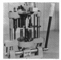
6. Rotate shell plate so that case with primer, powder, wads and shot is in station #5. Place empty case, primer and wads in their respective places and move operating lever to full down and up positions.
