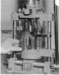
Move operating lever up to complete stop and remove loaded shell.
