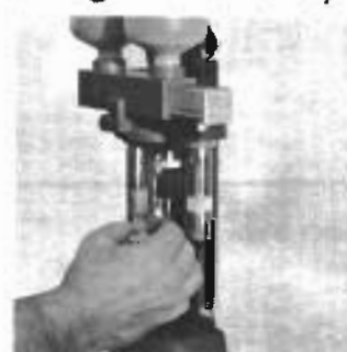
2. If you are using one-piece shot protector wads (such as Versalite) fit wad over powder/shot drop tube before lowering handle. If using fiber wads, place directly in wad guide. (Wad guide spring fingers may become damaged with extended use. To replace, break out damaged spring finger and snap in new unit from bottom of wad guide.)
