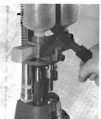
2. Lower operating lever to full "down" position. This seats new primer. (primer seating punch may be adjusted by loosening the lock nut and turning the punch to raise or lower it.)
