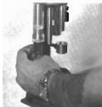
1. Insert empty shell case into die.
