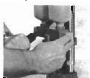
4. Raise handle slightly and move charge bar fully to left. This drops measured amount of shot into shell case. (Note: There should be about 1/2"-9/16" between the shot and the mouth of the case for proper crimping. If measurement is otherwise, you may be using the wrong combination of components.)
