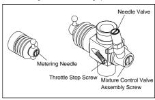
NOTE: Readjustment may be necessary, occasionally to allow for changes in fuel formula gear ratio or clutch engagement point.
