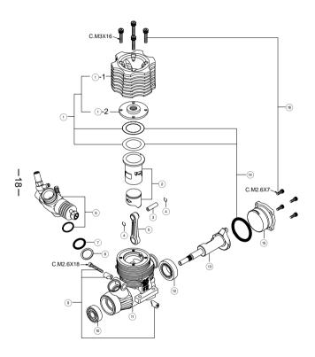
\* Type of screw C···Cap Screw M···Oval Fillister-Head Screw F···Flat Head Screw N···Round Head Screw S···Set Screw
