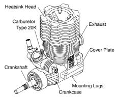
The engine is fitted with one each of 0.1mm and 0.2mm cylinder-head gasket when leaves the factory. Another 0.1mm head gasket is supplied with the engine. You may addit at initial runningin, when a glow plug tends to burn out due to high temperature and / or high humidity or when you prefer fuel economy to power.
