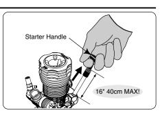
Do not attempt to disassemble the recoil starter. If you do so, the very strong spring inside will be suddenly ejected. This can be very dangerous.
