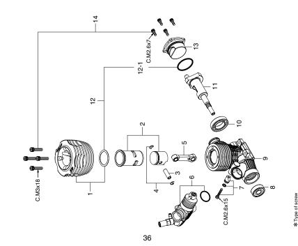
\*Type of screw C...Cap Screw M...Oval Fillister-Head Screw F...Flat Head Screw N...Round Head Screw S...Set Screw
