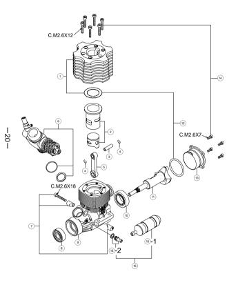
\*Type of screw C····Cap Screw M····Oval Fillister-Head Screw F····Flat Head Screw N····Round Head Screw S····Set Screw
