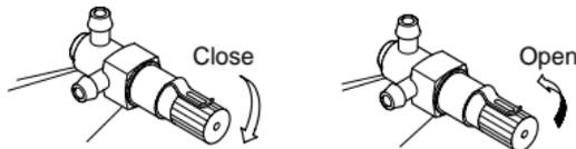
The position where the needle-valve stops is the fully closed position. It may be convenient to remember the position of the mark or set-screw at this time.
