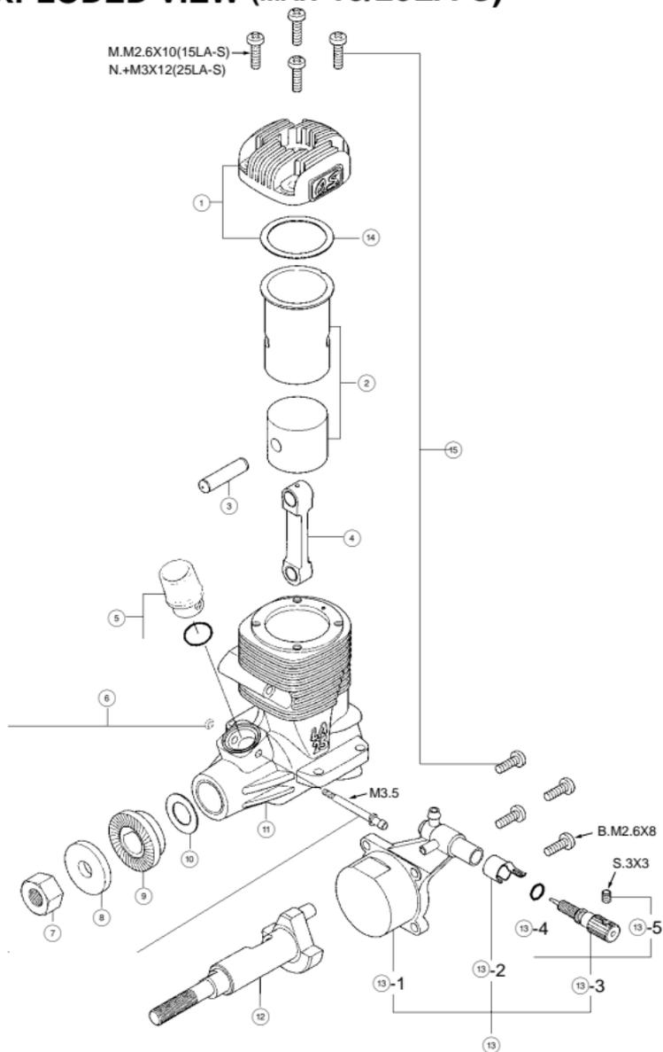
\* Type of screw C··Cap Screw M··Oval Fillister-Head Screw
