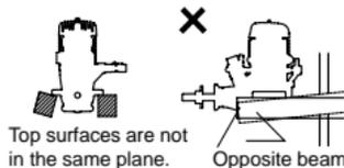
Re-align the surfaces as necessary
