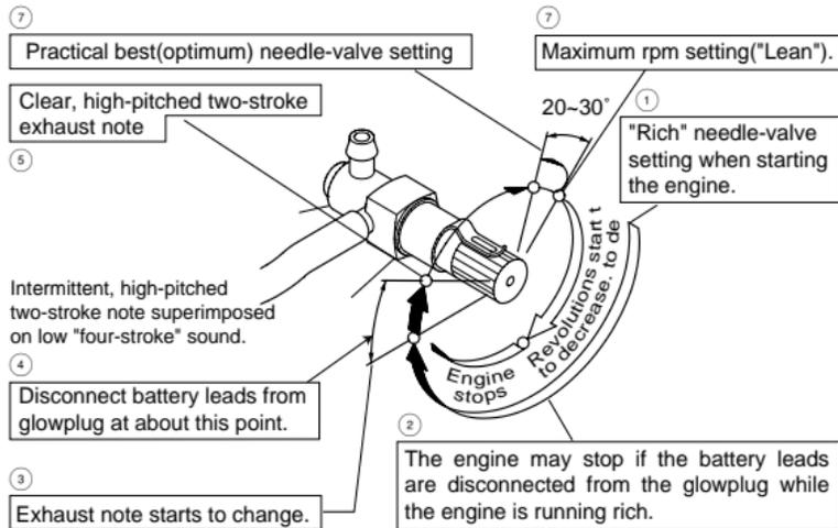
( Note: Although this is a two-stroke engine it fires like a four-stroke at these rich needle-valve settings-i.e. ignition of the fuel charge takes place at every fourth stroke of the piston instead of at every second stroke.
