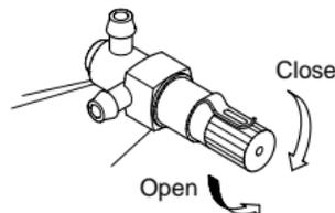
Turn needle-valve clockwise to close (for leaner mixture).
