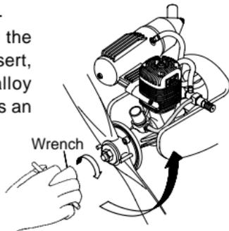
**Warning:** When using a spinner assembly, make sure that the notches in the spinner shell are large enough to clear the propeller blades and so do not cut into and weaken the blade roots.
