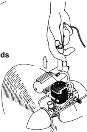
If the engine stops when battery leads are disconnected, close the needle-valve a little (approx. 45°) further, and restart the engine.
