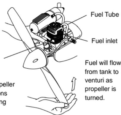
Turn the propeller two revolutions while watching the fuel line.
