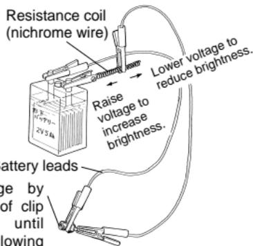
Adjust applied voltage by changing the position of clip on resistance coil until glowplug element is glowing bright red.
