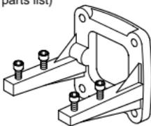
**Make sure that the mounting beams are parallel and that their top surfaces are in the same plane.**
