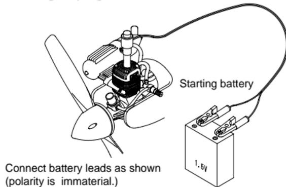
Connect battery leads as shown (polarity is immaterial.)
