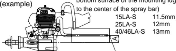
Measurement A (height from the bottom surface of the mounting lug to the center of the spray bar)
