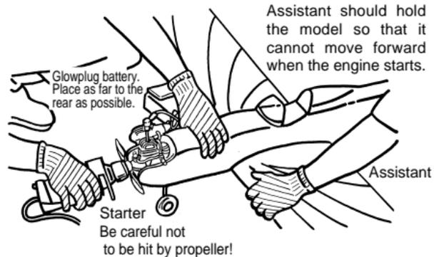
Assistant should hold the model so that it cannot move forward when the engine starts.
