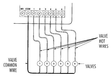
Connect the one common wire (usually the white strand) to the terminal labeled "COM". Connect the second "hot" wire (usually the color-coded strand) from each valve to one of the terminals numbered 1-6 on the number of stations on your timer model. Connect wire from valve 1 to terminal 1, valve 2 to terminal 2, etc.
