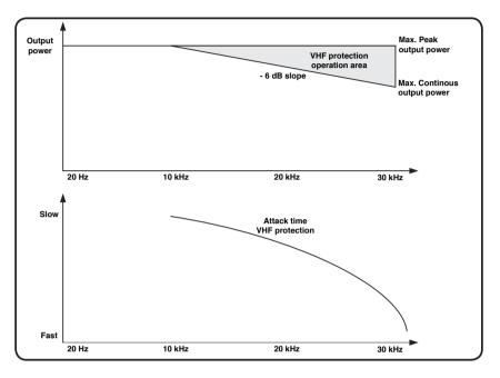
The Attack time for the VHF protection is increasingly shorter at higher frequencies. For example, an ultrasonic continuous signal will cause the outputs to mute rapidly, where it will take several milliseconds for a 10 kHz continuous signal to trigger the output mute. This is shown in the illustration above.
