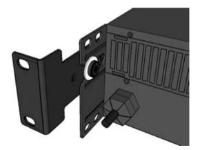
Figure 5.2b: Use washer for fixed installation
