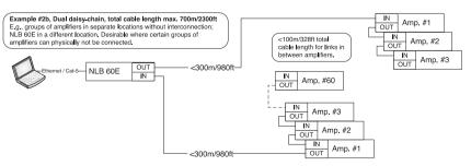
Figure 7.7.5d. NomadLink dual daisy chain closed loop configuration
