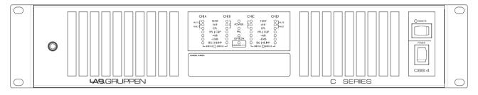
The amplifier's front panel presents the performance and fault condition indicators, power and remote switches, and a removable dust-filter cover. Four level potentiometers located behind the cover provide individual attenuation for the four amplifier channels. Range is 0 dB to - infinity. The 12 o'clock position indicates -10 dB attenuation. A label area is located beneath the LED display.
