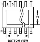
M24.173B 24 LEAD THIN SHRINK SMALL OUTLINE EXPOSED PAD PLASTIC PACKAGE
