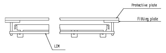
(2) When assembling the LCM into other equipment, the spacer to the bit between the LCM and the fitting plate should have enough height to avoid causing stress to the module surface, refer to the individual specifications for measurements. The measurement tolerance should be 0.1mm.
