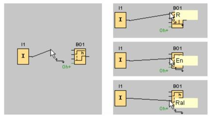
To make it easier for you to interconnect blocks, a blue frame around the mouse pointer pops when it is "captured" by a pin.
