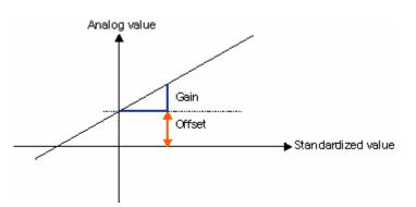
The straight line in the graphic describes which standardized value is being converted into which analog value. Gain corresponds to the slope of the straight line and offset to the movement of the zero passage of the straight line on the y-axis.
