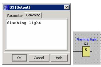
If you select a block with an associated label, the text is not marked. However, when you move the block, you also move the label. When you copy or cut the block, only the block itself is copied to the clipboard. A cut operation deletes the associated label. However, the associated label can be selected and moved, copied, cut or pasted individually. An associated label that is pasted from the clipboard is no longer associated with the block.
