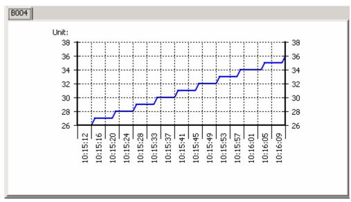
If your circuit program has more than one PI controller function block, the trend view has a separate tab for each PI controller analog output.
