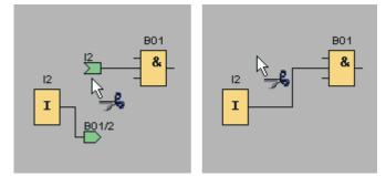
You should not use this tool to edit smaller circuit diagrams. In most cases you can optimize the layout by repositioning the icons.
