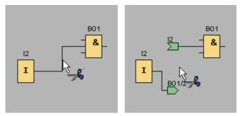
The connection is closed again by clicking on its open end while the Cut/Join tool is active. Optionally, you can close the connection by right-clicking on an open end and calling the **Link** menu command.
