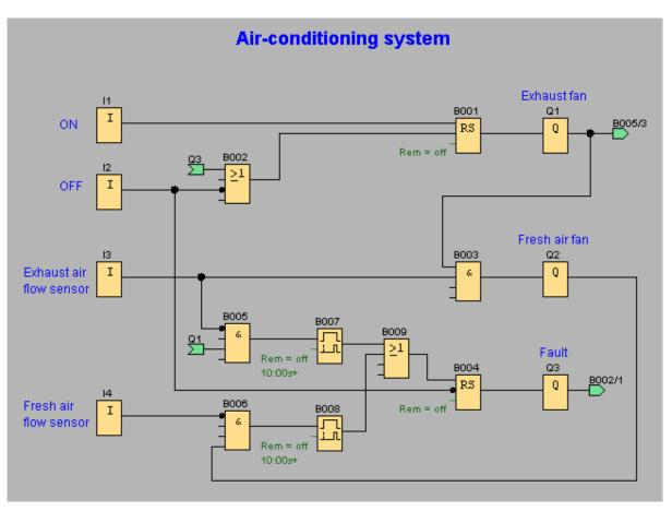
You can invert output Q3 to use output messages at Q4. Relay Q4 only drops out if main power is lost or if there is a fault in the system. The output can then be used for a remote message.
