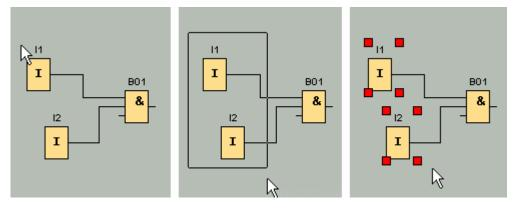
In addition to the selection of single objects by a simple mouse click or highlighting object groups by "capturing", there is a further selection option: Under "optional selection", mark the objects one after the other by holding down the [Ctrl] key while you select the objects. To remove an object from the selection, hold down the [Ctrl] key and click on a selected object once again.
