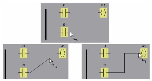
WindLGC offers you a further option of connecting blocks when you right-click on the input or output of a block. In the shortcut menu, click the **Connect to block** menu command. This calls a selection list that contains all blocks available for your connection. Click on the relevant target block. WindLGC then draws the connecting line. This method is especially useful for connecting a source to a target block over a greater distance on the programming interface.
