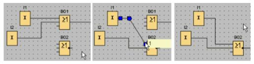
By keeping to this block replacement order, you can maintain your connecting lines. If you first delete the old block, you also delete its connections, which means you have to recreate all connections.
