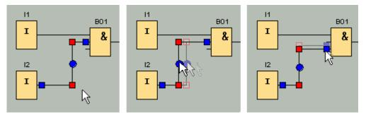
If the end of a connecting line is not assigned to a suitable target connector, it is automatically reconnected to its initial position after you "release" the mouse button.
