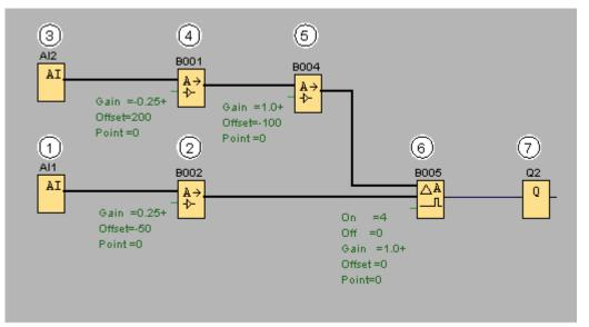
(1) A PT100 sensor is connected to an AI1, and this measures the lead temperature.
