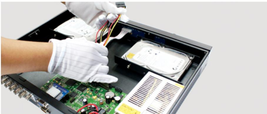
⑥ Use SATA cable connect to the DVR main board SATA ports, and then connect power cord to the HDD
