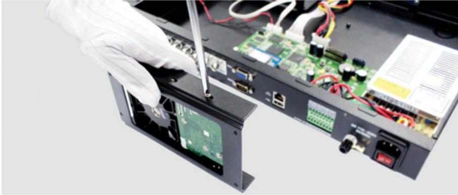
④ Fix the HDD bracket on the DVR base plate
