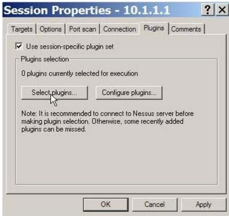
Figure 5: Selecting plug-ins with the Windows NessusWX Client
