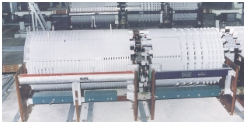
Fig. 24 Adjustable current limiting reactor
