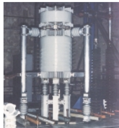
Fig. 25 Short circuit test reactor
