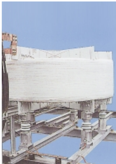
Fig. 20 Air core, encapsulated winding design
