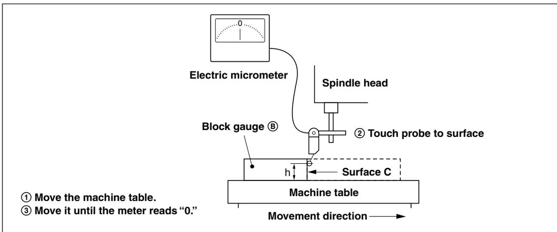
Note: Do not change the probe height h until finished measuring.
