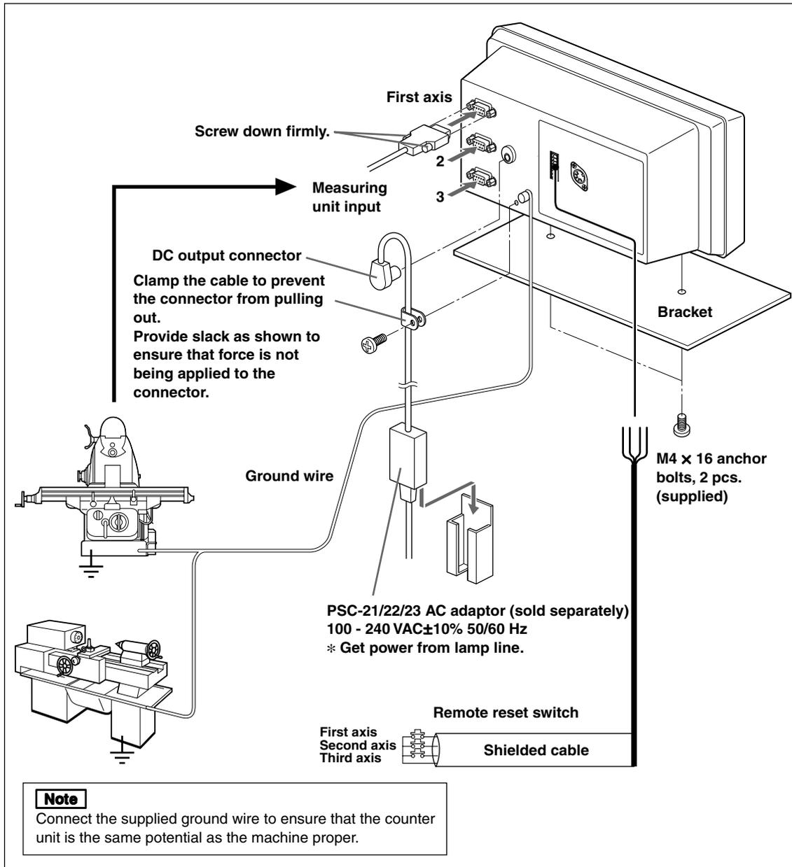
**Connections when using the addition function with lathe function**
