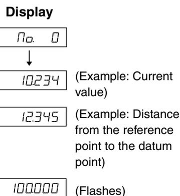
**<Inputting/restoring the reference point offset>**
