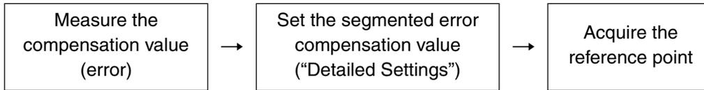
When the segmented error compensation value is set, the unit automatically switches to reference point acquisition mode after the detailed settings are finished, the power is turned on, or an error is reset. (See Part 7-2-9, “Reference Point Mode (How to Use the Measuring Unit with a Reference Point)”.)
