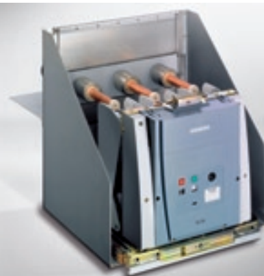
SION slide-in module completely prefabricated with circuit-breaker in cartridge, with insulating bushings and shutters – for simple integration of a circuit-breaker compartment in a switchgear bay
