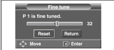
*If the reception is clear, you do not have to fine tune the channel, as this is done automatically during the search and store operation. If the signal is weak or distorted, you may have to fine tune the channel manually.*
