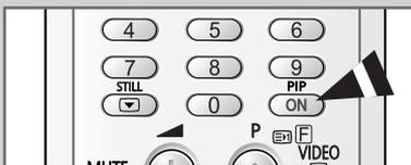
*You can display a sub picture within the main picture of TV program or external A/V devices. In this way you can watch TV program or monitor the video input from any connected devices while watching TV or other video input.*
