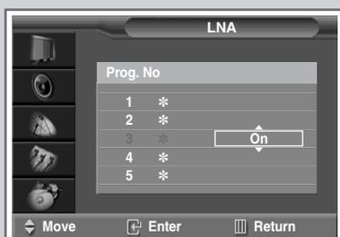
*This function is very useful in the situation that the TV is used in weak signal. LNA amplifies the TV signal in the weak signal area, but not noise.*
