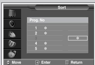
*This operation allows you to change the programme numbers of stored channels. This operation may be necessary after using auto store. You can delete the channels you do not want to keep.*
