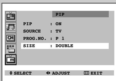
You can display a "Picture-In-Picture screen" within the main picture of TV program or Video input. In this way you can watch or monitor TV program or the Video input from any connected equipment while watching TV or other Video input. For information about connection of other equipment, see pages 42~43.
