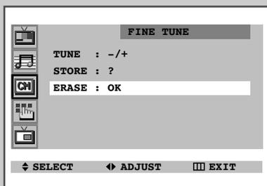
*If the reception is clear, you do not have to fine-tune the channel, as this is done automatically during the search and store operation. If however the signal is weak or distorted, you may have to fine-tune the channel manually.*
