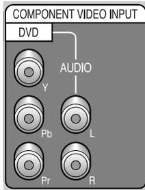
➤ The DVD/RCA (AUDIO-L and R) connectors are used for equipment with a DVD output.
