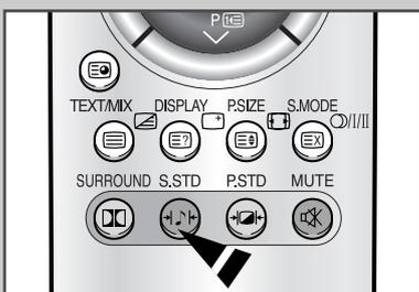
*You can select the type of special sound effect to be used when watching a given broadcast. The following sound effects are available in the order given:*
