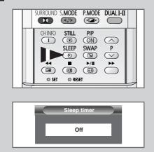
You can select a time period of between 30 and 180 minutes after the television automatically switches to Standby mode.
