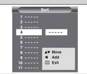
This operation allows you to change the programme numbers of stored channels. This operation may be necessary after using auto store. You can delete the channels you do not want to keep.
