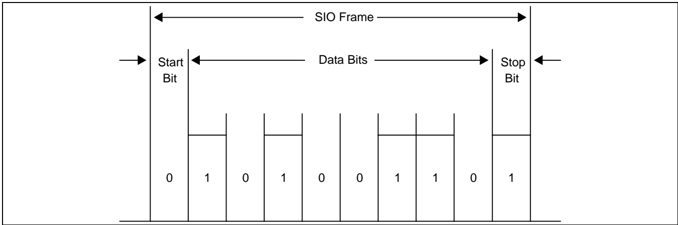
Figure 15-5. Serial I/O Frame Timing Diagram (Normal UART)
