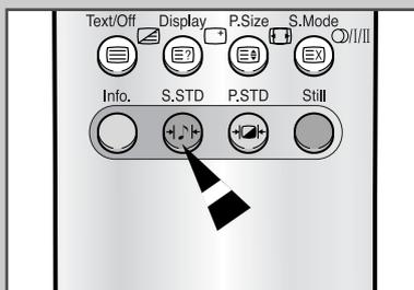
You can select the type of special sound effect to be used when watching a given broadcast.
