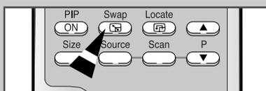
You can display a sub picture within the main picture. In this way you can monitor the input sources from any connected equipment.
