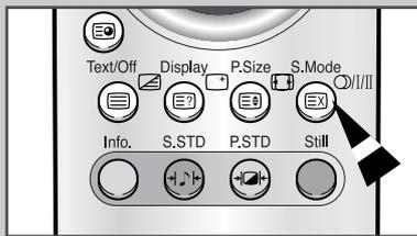
Depending on the particular program being broadcast, you can display and control the processing and output of the audio signal. When power is switched on, the mode is automatically preset to either "Dual-I" or "Stereo", depending on the current transmission.
