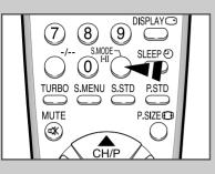
The "S.MODE I-II" button displays/controls the processing and output of the audio signal. When power is switched ON, the mode is automatically preset to either "Dual-I" or "STEREO", depending on the current transmission.
