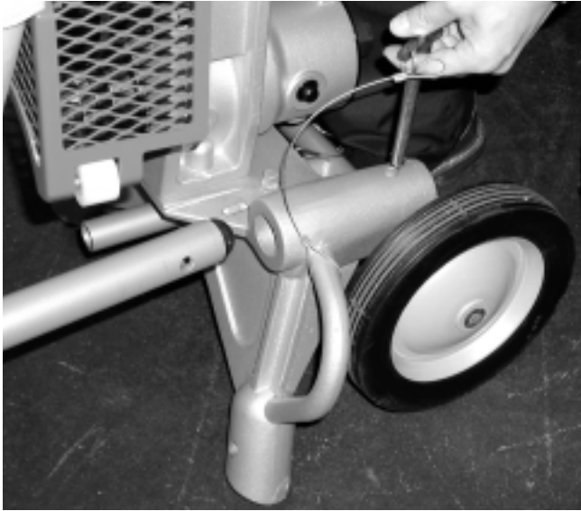
Figure 25 – Attaching the Support Legs
