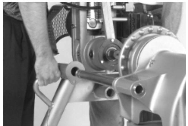
Figure 4 – Sliding Roll Groover Onto Support Arms
