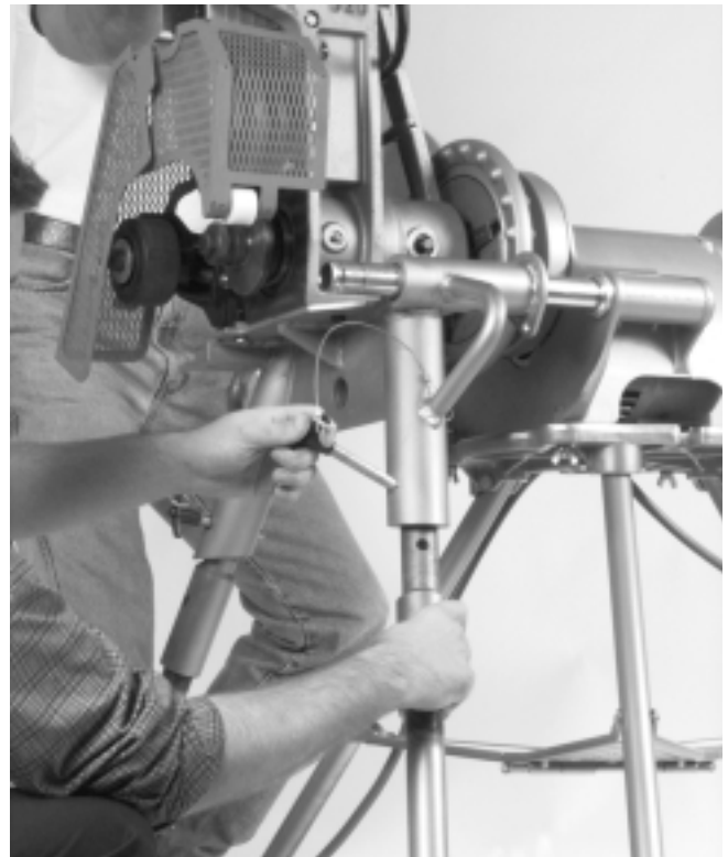
Figure 23 – Removing Legs From Base
