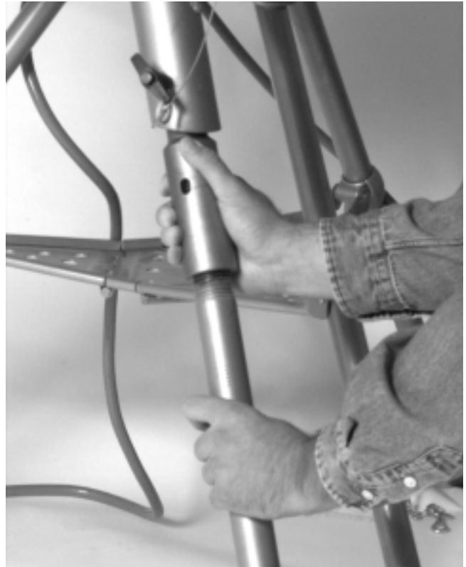
Figure 6 – Adjusting Legs to Level Groover
