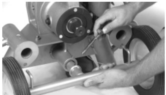
Figure 24 – Mounting the Groover to the No. 32 Transport Cart
