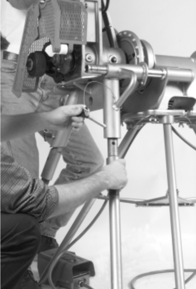
Figure 5 – Installing Legs Into the Groover Base
