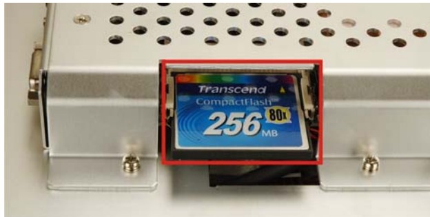
Figure 4-2: CF Card Installation
