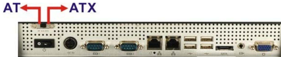
Figure 4-3: AT/ATX Switch Location
