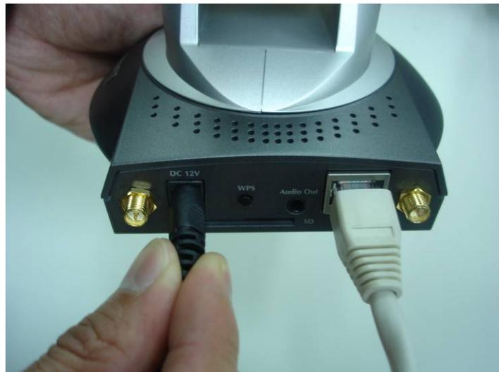
3. (ICA-M220W only) Connect two antennas to the antenna bases, which is located at the back of the PT Internet Camera.
