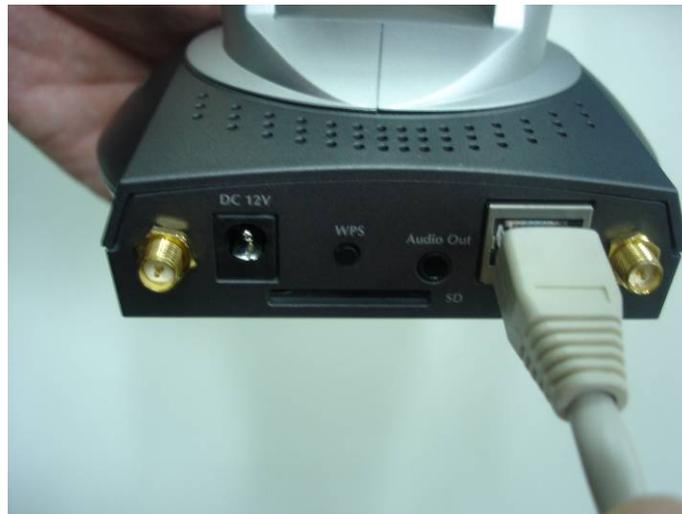
Plug the power adapter to wall socket, and connect the power connector to the power jack located at the bottom of the IP camera,
