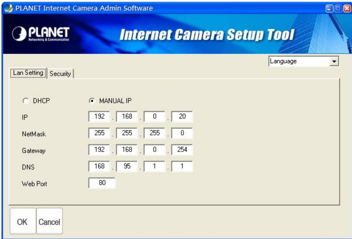
In **Lan Setting** page, user can configure camera's network settings. Select **DHCP** to set the camera to obtain an IP address from DHCP server on local area network automatically, and select **Manual IP** to input the IP address information manually. Click **OK** to save settings.
