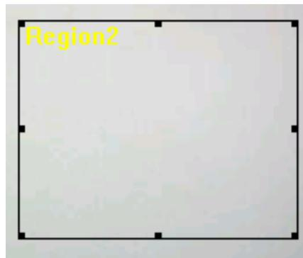
Move the mouse cursor to the eight dots located at the border of motion detection region, and the mouse cursor will switch to  $\leftrightarrow$ ,  $\nwarrow$  or  $\updownarrow$ . You can click and hold mouse button and move the mouse to resize the motion detection region.
