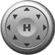
Moves camera to a new direction. Press one of 8 directional buttons to move the camera, and press **H** to move the camera back to 'home' (original) position.
