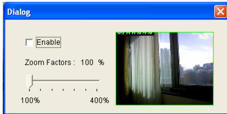
Click **Enable** to enable digital zoom function, then you can drag the slide bar to adjust zoom ratio. You can also use your mouse to drag the zoom area (the yellow square) to reposition the zoom area.
