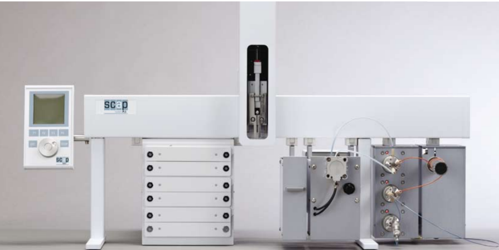
SCAP PLS system components mounted on a robotic platform
