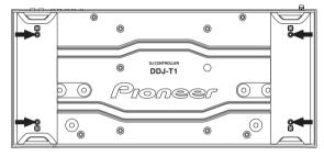
The screws you have removed will be needed when mounting the feet. Be careful not to lose them. The feet cannot be properly mounted using other screws.
