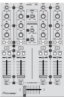
MAIN VOL control Adjusts the sound level output from the master.
