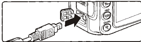
Connecting the GP-N10 to a D90 digital camera
