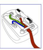
3. The BROWN wire must be connected to the terminal which marked with the letter "L" or coloured RED.
