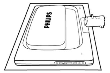
2) Hold the monitor base with both hands and firmly insert the base stand into the base column.
