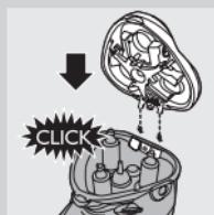
light starts to blink with intervals and the holder returns to its starting position. Refill the cleaning chamber with cleaning fluid up to the MAX indication (see chapter 'Cleaning and maintenance').
