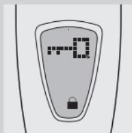
*Note: if you press the on/off button again within a few seconds after entering the travel lock mode, the travel lock will not be activated. Instead, you will have entered one of the two display layout modes. If you want to return to the travel lock mode, press the on/off button two more times until you are back in the travel lock mode (indicated by a rotating key symbol). Then wait a few seconds without pressing the on/off button to activate the travel lock.*
